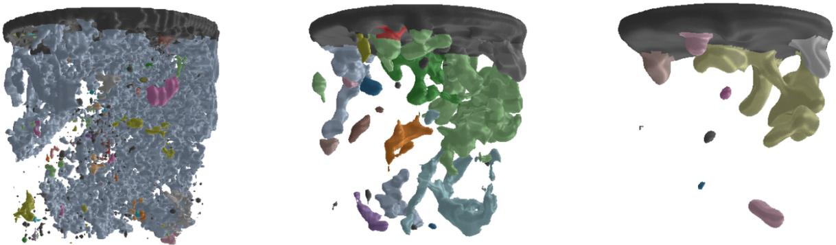
Figure 10: The effect of Gaussian smoothing on the density estimation. In (left) no smoothing is applied, in (middle) a smoothing kernel of size 1.0 is used, and in (right) a smoothing kernel of size 2.0. The low-pass filter is necessary for removing noise, however applying too large of a kernel reduces the structural detail of the resulting fingers.
