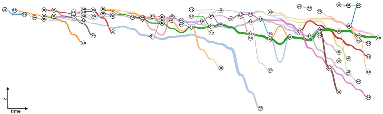
Figure 7: *Spatio-Temporal Reeb Graph* projected as a line chart where the  $x$ -axis is time, the  $y$ -axis is the average  $z$ -position of a finger, and line thickness encodes finger length. This projection is used to explore trends and identify outliers while also visualizing the evolution of fingers, i.e., the time they appear (discs), disappear (discs), merge (diamonds), and split (diamonds). For better readability the nodes are also labeled with their corresponding time step.
